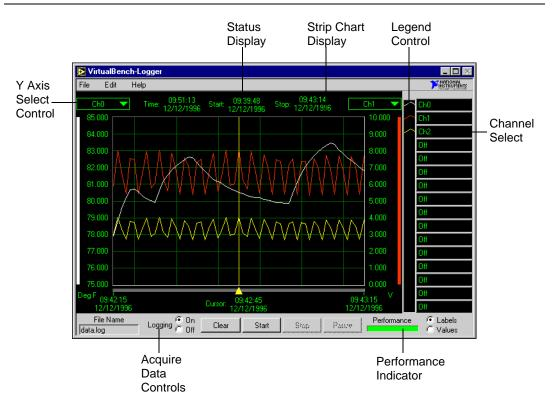
The front panel of VirtualBench-Logger has the following features:
